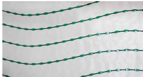
Example of a moisture management housewrap with 1.5 mm spacers that provide a drainage space between the sheathing and cladding material. Image provided by Tamlyn.
