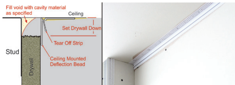
Ceiling mounted deflection beads also prevent inside corner ceiling cracking due to deflection in multi-story structures, but they are mounted to the roof deck, allowing the bead to slide up and down the wall during deflection.
