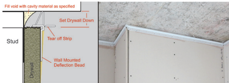
Wall mounted deflection beads are designed to attach to drywall and compress against the concrete deck during deflection to prevent inside corner cracking.
